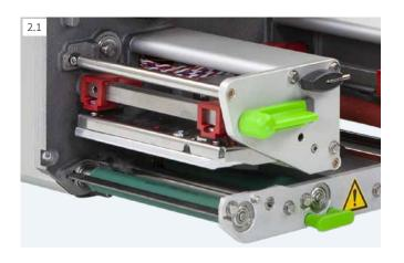
All print heads are freely interchangeable at equal width.
